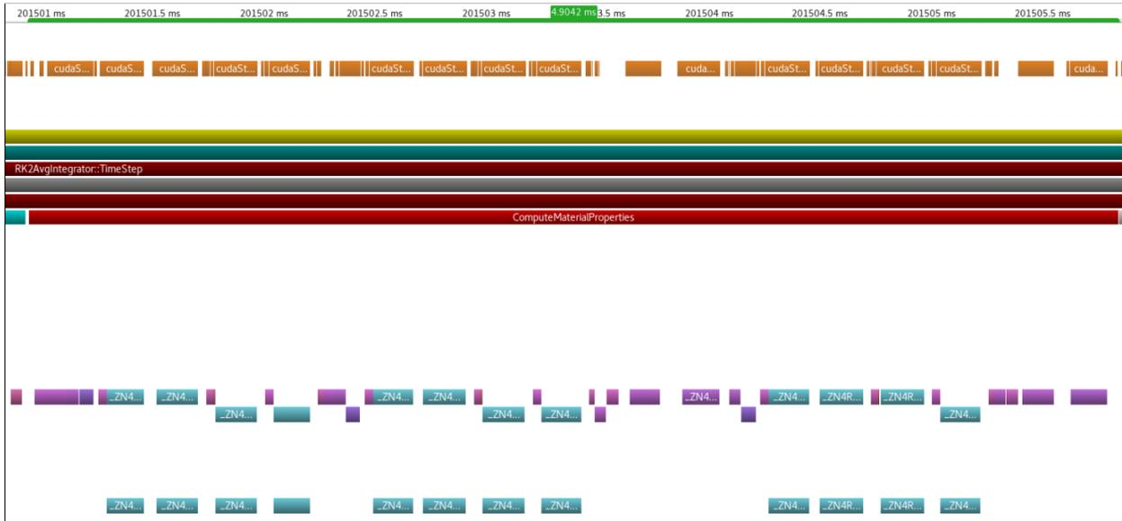
Figure 4: Screenshot from an Nvidia visual profiler (nvvp) session highlighting the breakdown of kernel calls within a single `ComputeMaterialProperties` annotation (red) in a 3-node run of the Shaped Charge Problem. The LEOS calls within this 5 millisecond interval are primarily in the blue blocks on the bottom row as well a subset of the smaller purple blocks. The larger purple blocks within this annotation include calls to MARBL’s material strength library Leilak.
